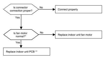
\* It is normal when check hall sensor of indoor fan motor as shown below
